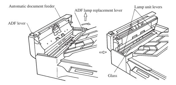
Figure 5.4 Lamp unit removal 1
